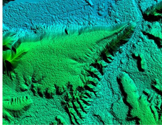
Figure 6. 2 m DTM derived from 50cm GeoEye-1 stereoscopic imagery viewed in Global Mapper
