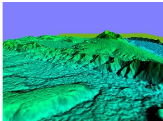
Figure 7. 2 m DTM derived from 50cm GeoEye-1 stereoscopic imagery. 3D view in Global Mapper
