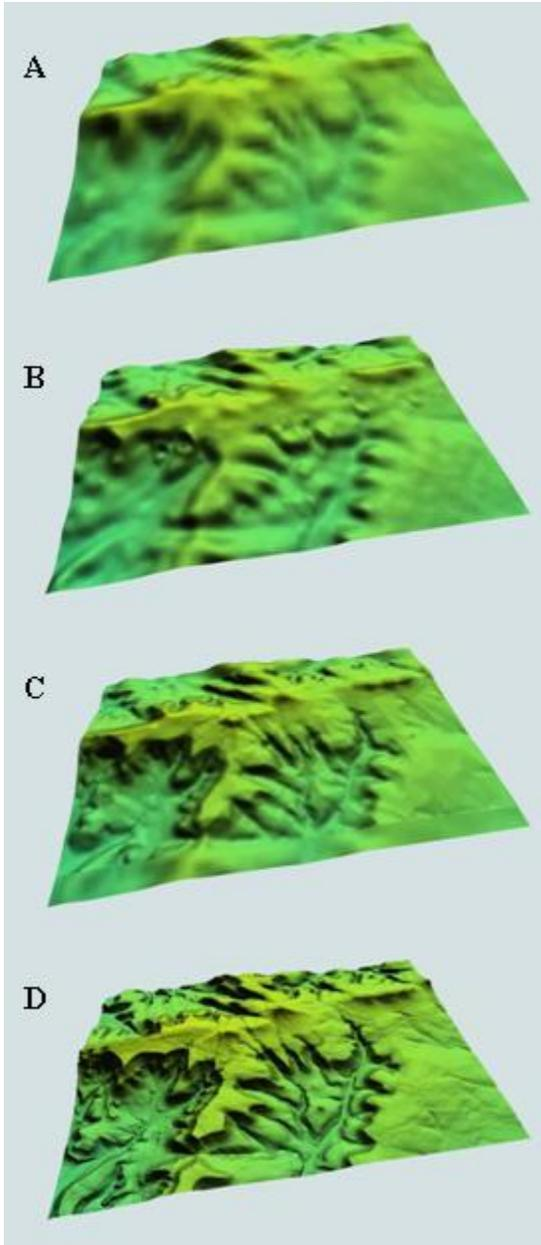
Figure 3. A. SRTM 90 m DEM. B. ASTER 30 m GDEM. C. Topographic 30 m DEM. D. GeoEye-1 3 m DTM.
