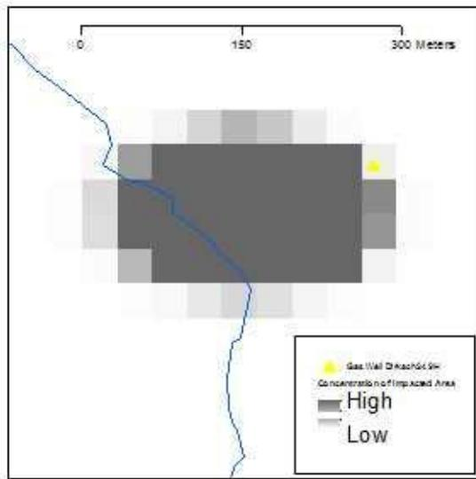
Figure 4. Porous Puff gridded area of contamination. Darker areas indicate greater concentration of contaminants.
