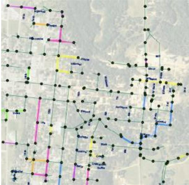
Figure 7. Zoomed in portion of the six-phase recommendation plan to televise and replace pipes. The yellow colored pipes signify the first year televising and replacement plan. The orange and pink colored pipes indicate phases 2 and 3, respectively. Phase 4 is depicted by the purple pipes, while the light blue and dark blue pipes represent phase 5 and 6.
