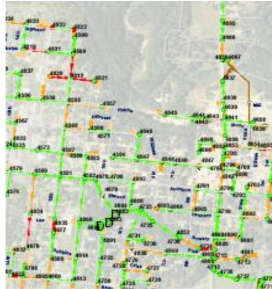
Figure 6. Zoomed in portion of the final GIS. Green pipes and manholes are structurally sound with positive flow. Orange and yellow manholes are not in immediate need attention, but should be considered in the long run of replacements. The red pipes have a negative slope and need immediate attention. The red manholes are structurally poor and require replacement.
