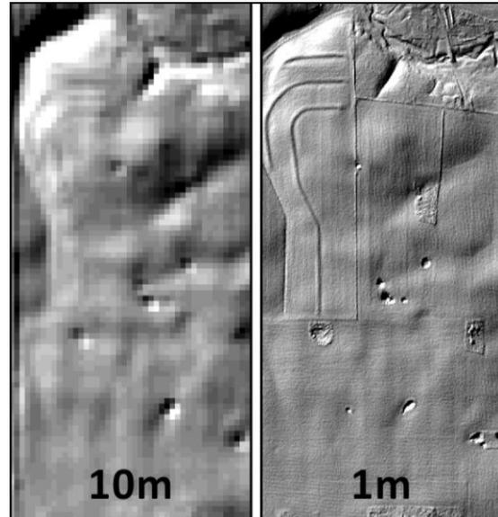
Figure 3. Resolution matters; the DEM on the left has 10 m (32.8 ft) resolution compared to 1 m (3.3 ft) resolution of the DEM on the right. Sinkholes and terraces on the left are much fuzzier and less recognizable compared to those same features on the right. The DEM on the right shows more detail and will yield greater model accuracy and thus more potential conservation value. Both images are at a common same scale of 1:12,000.
