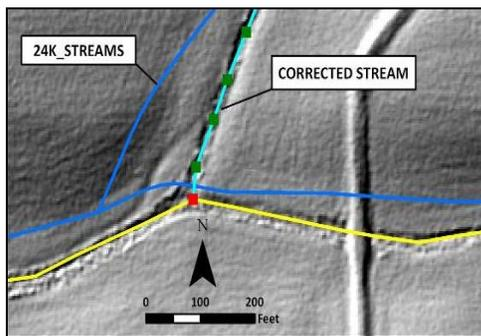
Figure 6. Corrected stream network in the study area using a hillshade layer for a reference.
