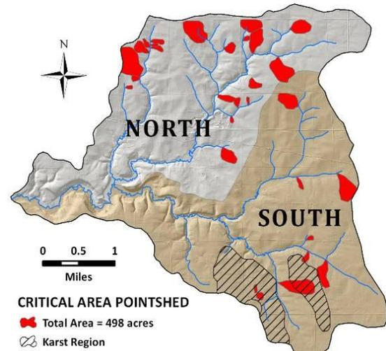
Figure 11. Distribution of critical area pointsheds in the Bear Creek study area. Of the 498 total ac, 334 ac (67%) were located in the northern half and the remaining 164 ac (33%) were located in the southern half where karst features occur.
