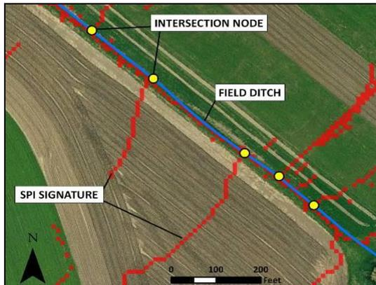
Figure 8. SPI signatures are shown in red identifying places where overland runoff and concentrated flow occurs. Yellow dots are places where a SPI signature intersected with field drainage ditch and potentially represents active erosional features.
