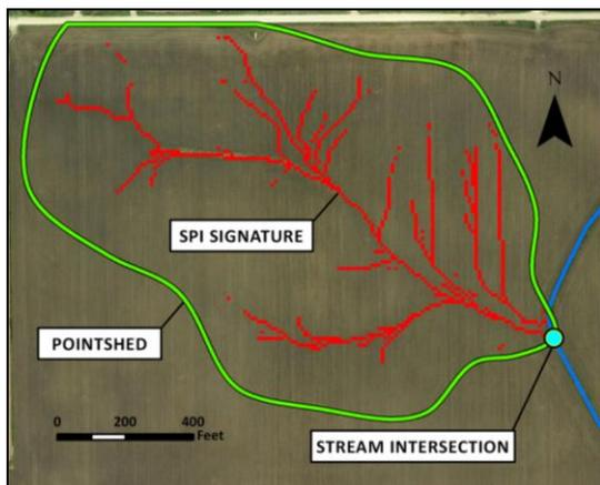
Figure 10. Pointshed delineated around the upslope contributing area for a critical area within the Bear Creek study area. The contributing area shown here measured approximately 30 ac.
