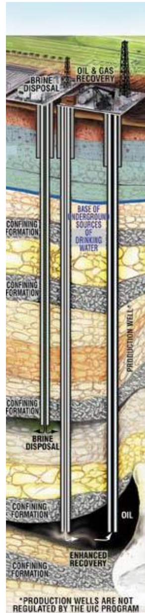
Figure 1. Diagram showing a production well and a class II injection well (Environmental Protection Agency, 2016). On the right side of the figure is the oil and gas production well and on the left a slightly shallower Class II disposal well where brine water and other fluids are injected underground.
