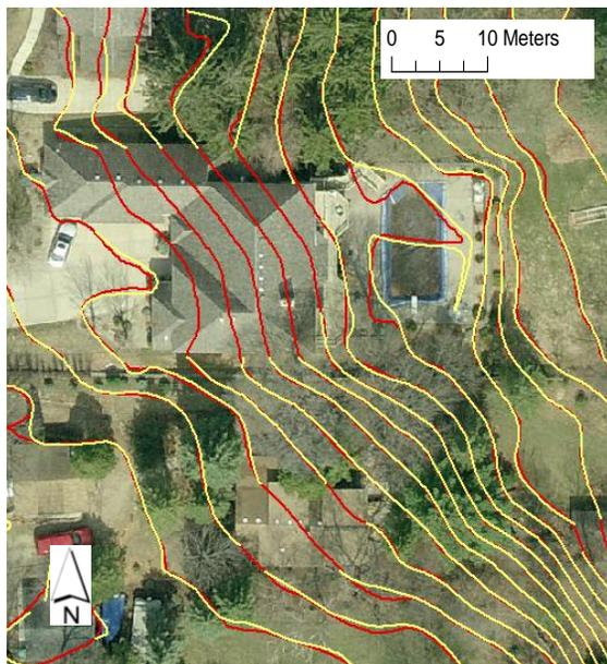
Figure 4. A comparison of Ramsey County contours (yellow) to contours derived from the terrain model (red).
