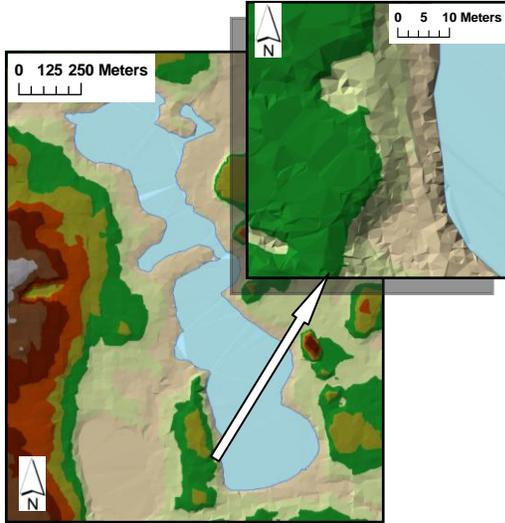
Figure 3. Terrain layer of the study area depicting resolution of 3rd pyramid level at 1:15,000 (lower left) compared to 1st pyramid level at 1:600 (upper right).
