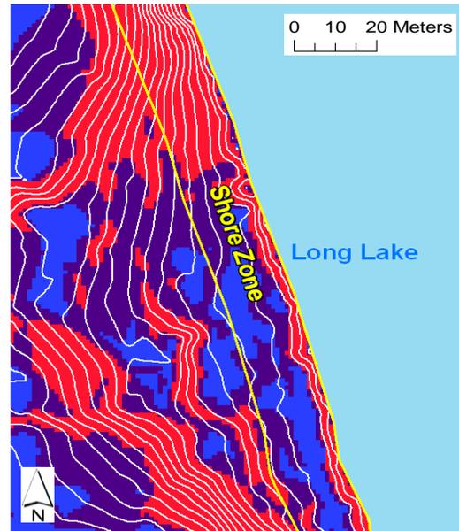
Figure 5. The reclassification of the slope grid with overlain contours for comparison. The slope ranks are depicted as Blue = 1 ( $\leq 10:1$  slope), Purple = 2 ( $>10:1 - 5:1$  slope), and Red = 3 ( $>5:1$ -Vertical slope).
