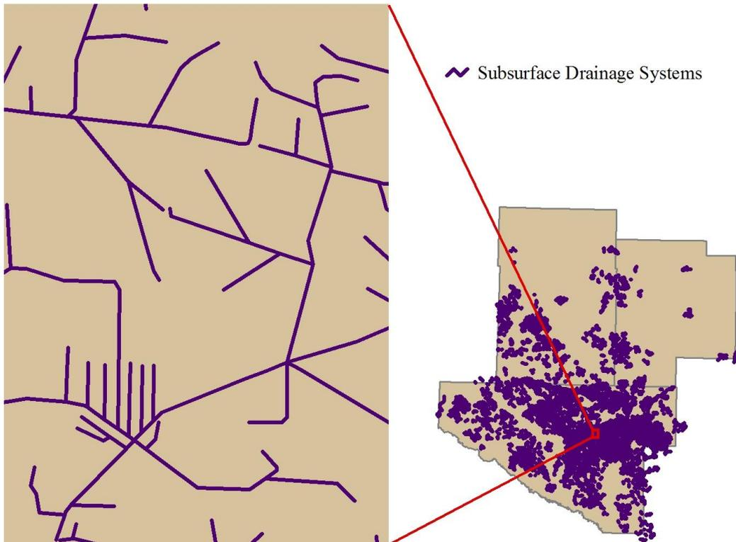
Figure 2. Subsurface drainage systems overview (right) and detail (left) in Kandiyohi, Meeker, and Renville Counties, MN. Purple lines indicate the locations of drain tile. The overview is shown at a scale of 1:1,750,000. The detail is shown at a scale of 1:24,000.
