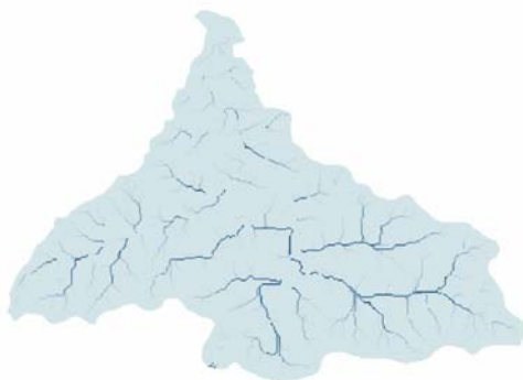
Figure 10. Flow accumulation grid (10 meter cell size).
