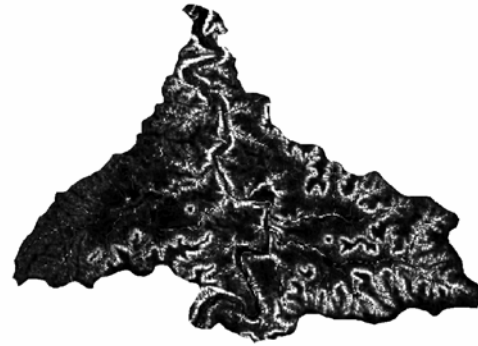
Figure 11. Slope length and steepness grid (10 meter cell size).
