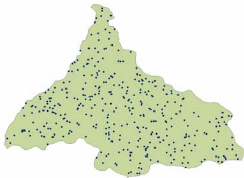
Figure 12. Random sampling points shapefile created by Hawth’s Analysis Tools.
