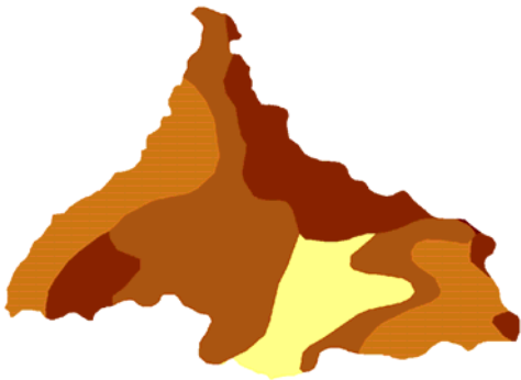
Figure 5. STATSGO grid (10 meter cell size) representing K factor (soil erodibility) values.
