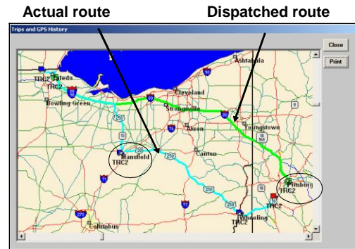
Figure 5. Plot route versus actual. Blue line represents actual route, Green line represents dispatched route.
