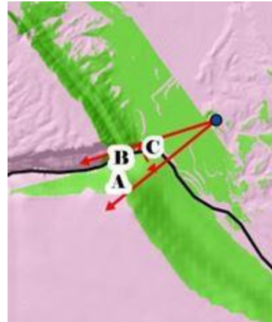
Figure 3. Santa Elena Canyon output viewshed created during this study (Green = visible), Location of Santa Elena Canyon Integral Vista (Blue Dot) Digital Elevation Model (Transparent Fuchsia) Prominent Features (Letters), Viewshed Angle (Red Arrows) and BIBE Park Boundary (Black Line).
