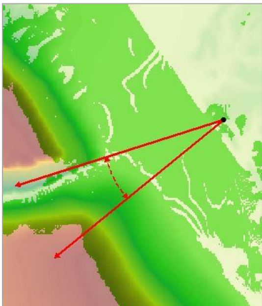
Figure 8. A portion of the viewshed Boolean raster output for Santa Elena Canyon Integral Vista (Black Dot) and visible area (Green).
