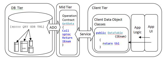
Figure 2. Application 2 n-tier diagram.
