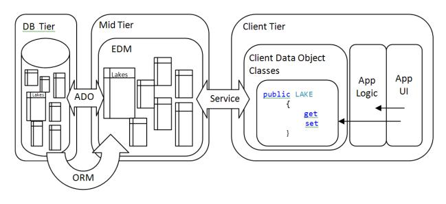
Figure 1. Application 1 n-tier diagram.
