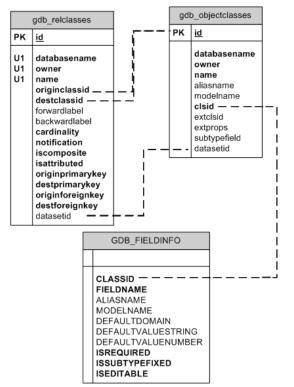
Figure 3. Geodatabase system tables used by Application 2.
