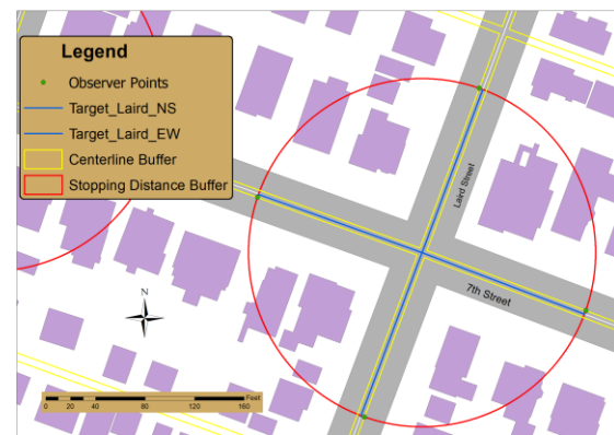
Figure 2. Diagram showing the principle components of the initial setup for the intersection of 7th and Laird streets. The components are the Stopping Distance Buffer (red), the Centerline Buffer (yellow), Observer Points (green) and the Target Lines (blue).
