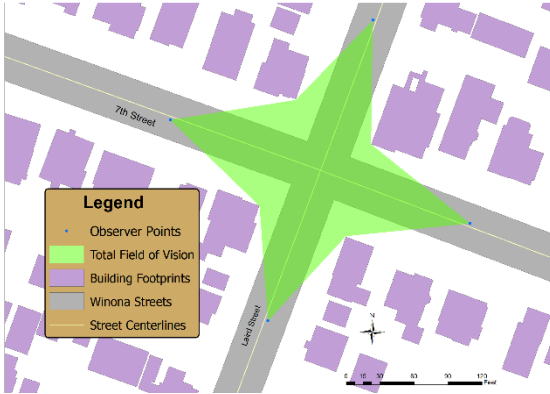
Figure 7. The diagram of the Intersection Total Field of View for the intersection at 7th and Laird. The Total Field of Vision is 187.47°.
