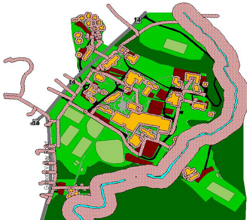
Figure 8. This map shows the model created to determine which land is occupied due to building codes and floodway limits.
