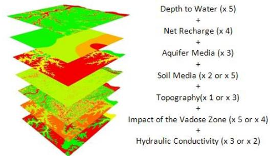
Figure 1. The procedure for calculating the DRASTIC index and the Pesticide DRASTIC index is multiplying the values of the raster layer by the weight and adding the weighted results.
