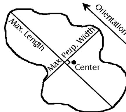
Figure 2. The parameters recorded by the ground survey to describe gap spatial characteristics.
