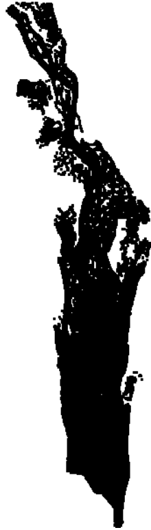
Figure 3. Land / Water boundary polygon shapefile digitized from the 1998 DOQ imagery showing the water polygon as black.
